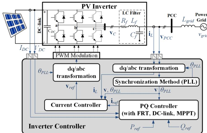
Figure 2: Grid tied inverter controller with its main units: park transformation, synchronization scheme, PQ controller and current controller.
