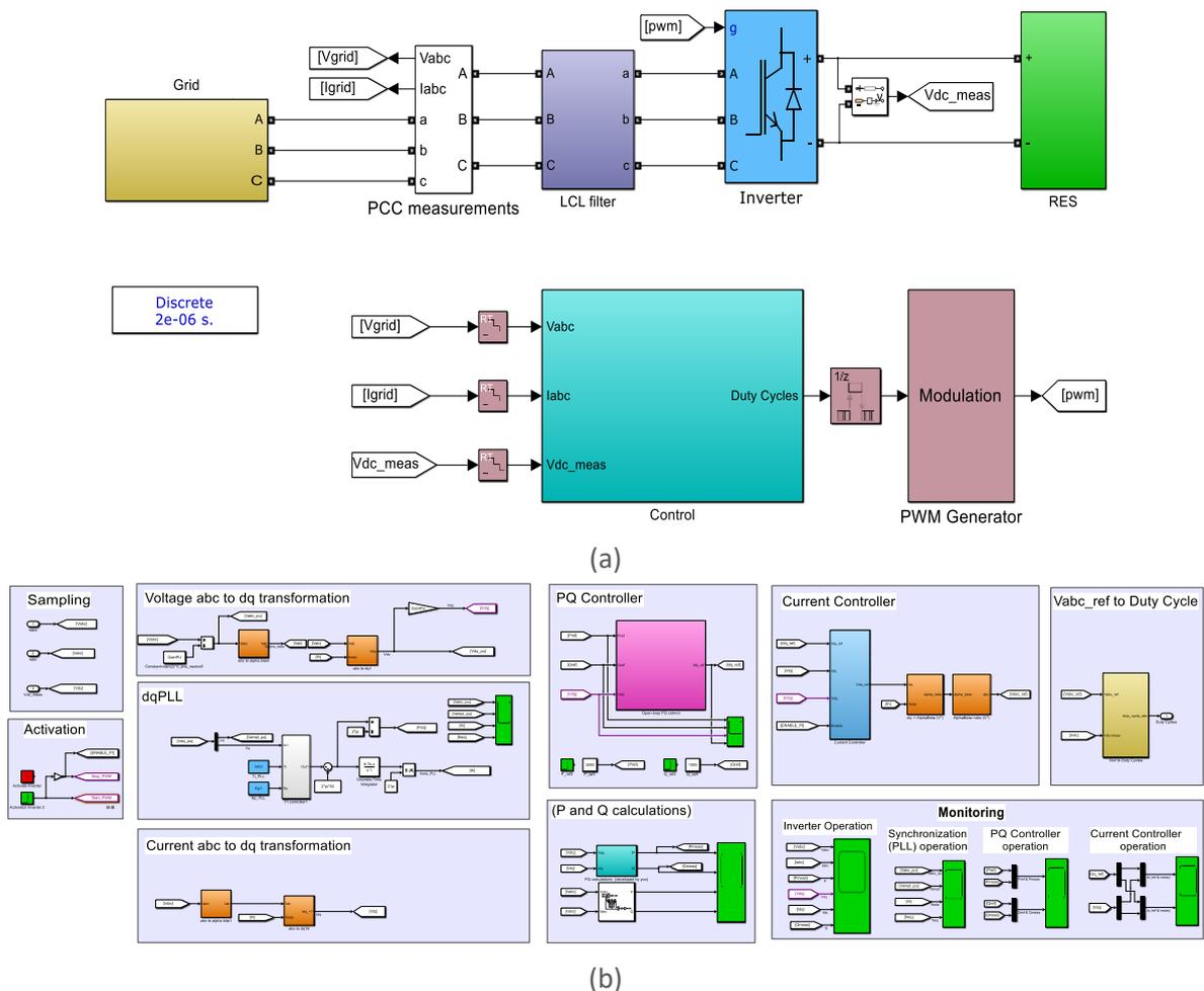
Figure 6: (a) Grid tied inverter model and (b) Inverter controller design in MATLAB/Simulink.
