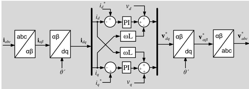
Figure 5: Structure of the conventional current controller.
