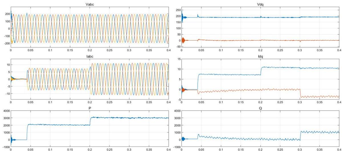
Figure 7: Inverter operation with step change on active and reactive power set-points.
