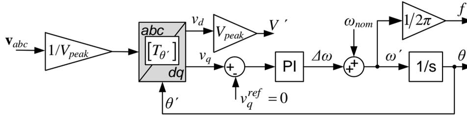
Figure 3: Synchronization unit design based on a PLL approach.
