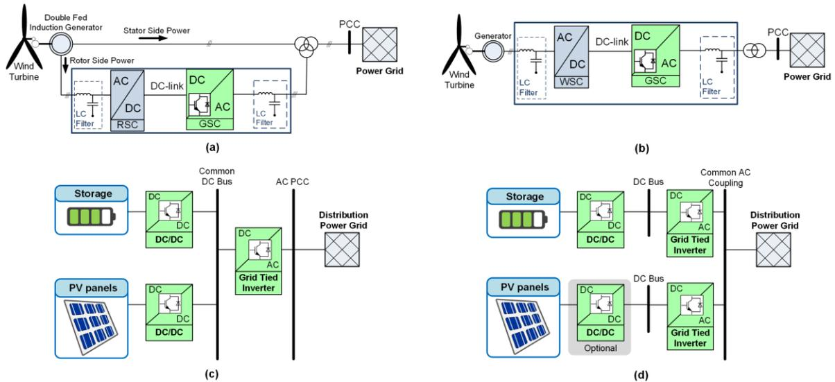
Figure 1: Power converter configurations for wind and PV-storage systems: (a) Wind turbine configuration based on double-fed induction generator and back-to-back power electronics converters in the rotor side of the generators; (b) Fully-converter wind power system where power electronics are handling the entire power flow; (c) DC coupling configuration for PV and storage systems based on a common inverter; (d) AC coupling configuration for PV and storage system with independent inverters.
