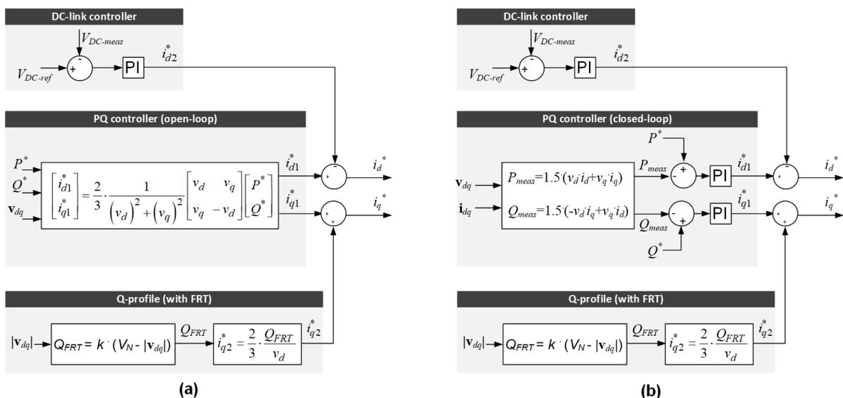
Figure 4: (a) Open-loop PQ controller, (b) closed-loop PQ controller.
